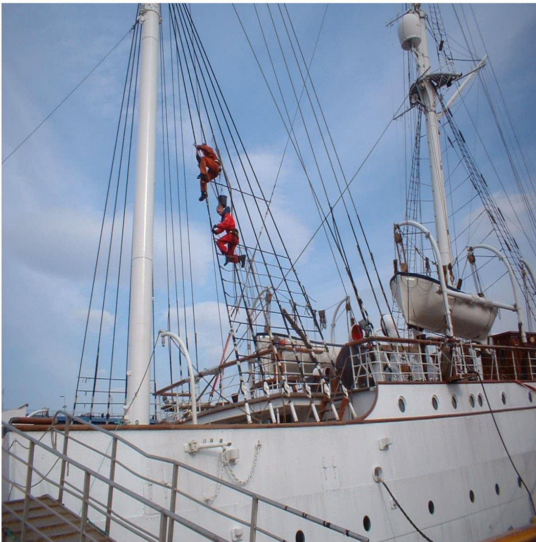
Making new ratlngbars and ratlines in Mainshrouds
